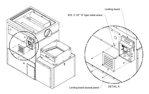
Limiting board installed on the left side of the furnace
