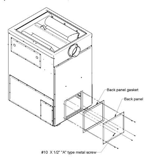
Remove the cold air ducting support from the cold air return box. To do so, remove the 12 screws as shown below. Keep these screws. You will need them to install the cold air ducting support in the new location.
