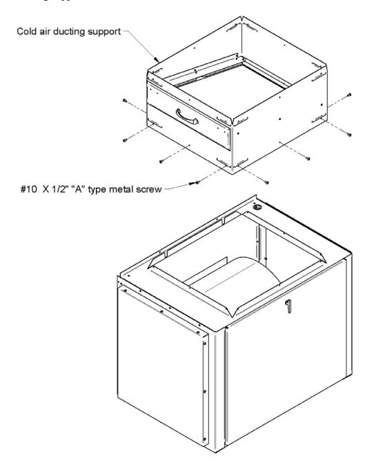
Then, secure the cold air return box to the furnace. To do so, use the 8 screws as shown below. Then, level the cold air return box by screwing or unscrewing the elevator bolts.
