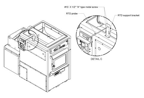
Once the RTD probe is installed on the RTD support bracket, you need to connect the RTD probe to the limiting board. To run the wire properly, refer to the drawings below. Refer to the electric wiring diagram in the owner's manual of the furnace for the electrical connections.
