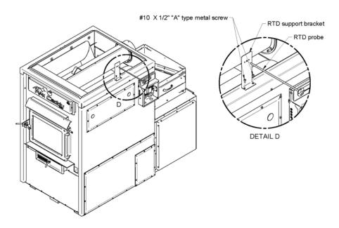
RTD support bracket installed on the LEFT side of the furnace
