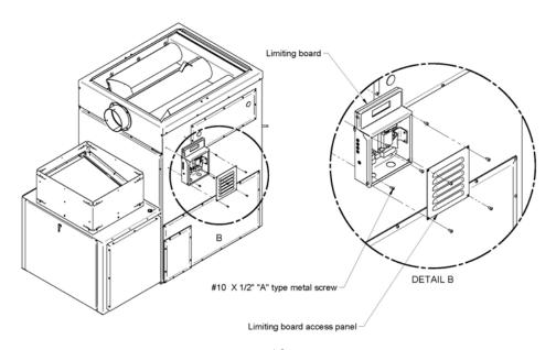
Now, it is time to make the connection between the limiting board and the blower. Since the limiting board may be installed on either side of the furnace, refer to the drawings below to run the wire properly.
