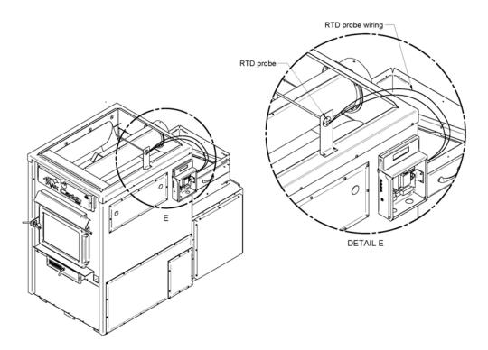
RTD probe installed on the **LEFT** side of the furnace
