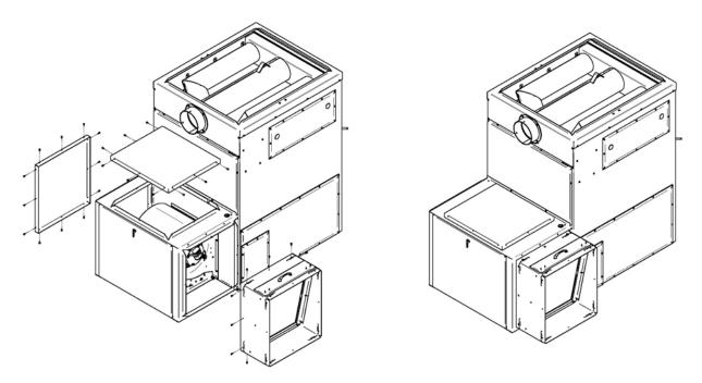
Installation of the cold air ducting support **ON TOP** of the cold air return box with filter exit towards the **RIGHT**
