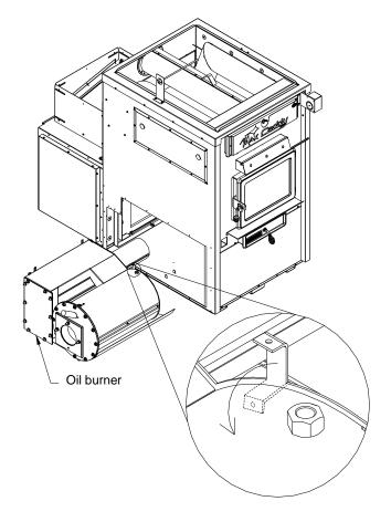
Step 7: Install the gasket on the left panel. The gasket is supplied with the oil unit option.
