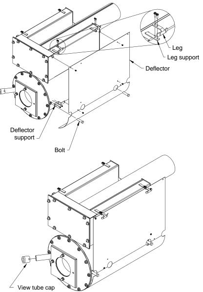
Step 2: Remove the view tube cap. In order to do so, partially unscrew the screw maintaining it in place.
