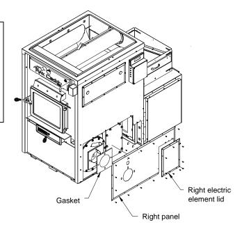
Step 8: Put the view tube cap back in place. Install the oil unit using nuts and washers supplied with the option as shown on the right. It is important to stick the certification label next to the unit.
