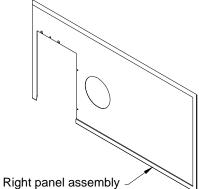
Step 11: Secure the right panel using the screws. Secure the right electric element lid back in place. It was removed in Step 5.
