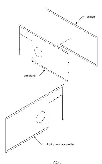
Step 10: Secure the left panel using the screws. Secure the left electric element lid back in place using the screws that you kept from Step 4.
