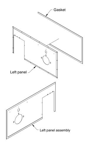
Step 8: Before installing the left panel, put the gasket on the oil unit. Secure the left panel using the screws. Secure the left electric element lid back in place using the screws you kept from Step 4.
