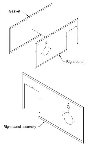
Step 7: Before installing the right panel, put the gasket on the oil unit. Secure the right panel using the screws. Secure the right electric element lid back in place using the screws you kept from Step 3.
