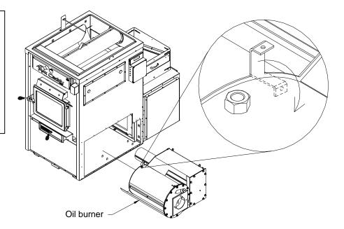
Step 6: Install the gasket on the right panel. The gasket is supplied with the oil unit option.
