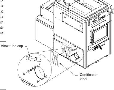
Step 10: Install the gasket on the right panel. The gasket is supplied with the oil unit option.
