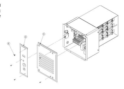
Once the wiring as per **Appendix 1** is completed, slide the electric element assembly (F) into the left hand side opening in the furnace cabinet.
