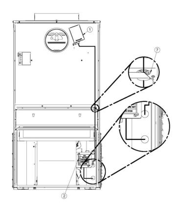
Run an 18-2 cable (not supplied) from the thermostat (3) included with your furnace through the top opening made in **Step 6**.
