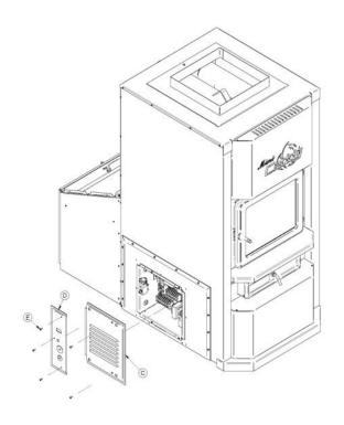
Install the fan limit control (G) supplied with the electric element. Remove the control's cover. Slide the control's probe in the opening located in the upper right corner next to the flue outlet. Secure the fan limit control with the screws (not supplied) in the holes intended for this purpose. Put back the control's cover.
