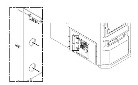
Using a flat screwdriver, remove the largest knockout located on the left access panel of the electric element.
