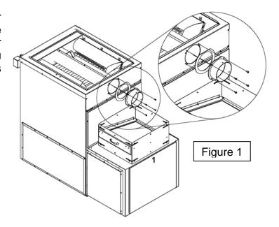
**Step 2**: Remove the four screws already installed on the cold air plenum support exhaust pipe. Keep these screws.
